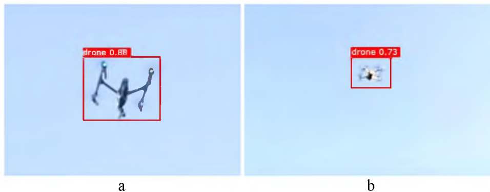
Figure 5. Frames from the inference of the trained YOLOv9c model: a) frame from the video of the DJI Inspire 2 flight; b) frame from the flight of the DJI Mini 3
