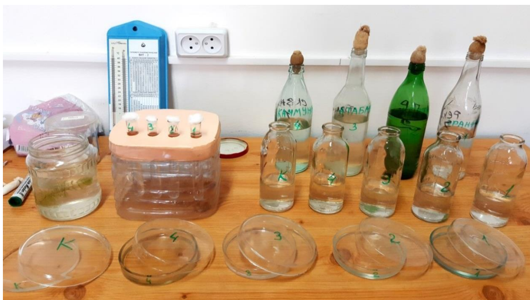
Figure 2-the course of the experiment, the degree of toxicity of wastewater using the Daphnia Magna test object
